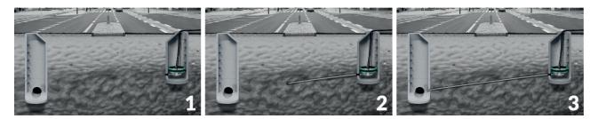
2. The next pass, we drill through the exit manhole wall and then, behind the reamer, we pull in the PP pipeline modules. The subsequent modules are attached by means of a hydraulic pipe assembly tool.
